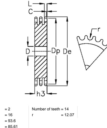
C = 2 D = 16 De = 93.6 Dp = 85.61 For chain size =  $3/4 \times 7/16$ For chain type = 12 B-3 h3 = 49.8 L = 10.8
